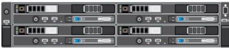
Figure 4. Front View with Server Modules
